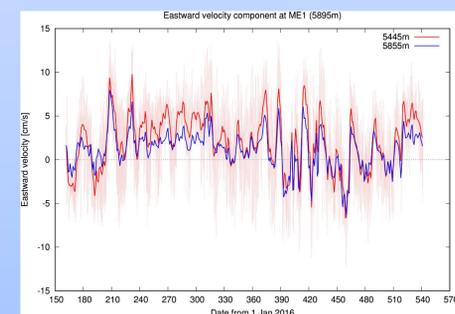
**Fig. 8.** Time-series of low-passed eastward current velocity at 40-m (blue) and 450-m (red) height from the bottom at ME1. Thin pink line shows hourly data including tides.
