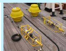
**Photo.** Current meters FSI 3D-ACM, major instruments of the mooring systems.
