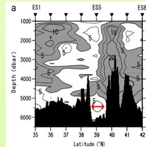
**Fig. 4.** Eastward velocity component (cm/s) section at 170E including Main Gap (shown by red arrow) by LADCP observation in R/V Hakuho Maru KH-03-1 Cruise (Komaki and Kawabe, 2009)
