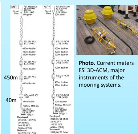
**Fig. 6.** Mooring systems deployed at Main Gap (ME1 and ME2). "450m" and "40m" are heights from the bottom, where current data were recovered and analyzed in this study.
