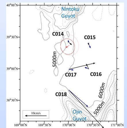
**Fig. 7.** LADCP bottom-tracked current vectors and Current Meter mean current vector in Main Gap. Black and blue arrows show near-bottom and 15-m height LADCP vectors, and red and pink arrow shows 40-m and 450-m height CM vector, respectively.
