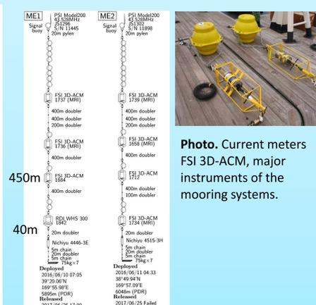
**Photo.** Current meters FSI 3D-ACM, major instruments of the mooring systems.
